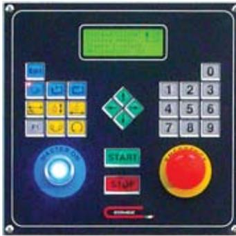
*Easy touch pad controls have many programmable features such as pause, speed and timing sequence.*
