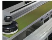
The **cupslide** allows for longer images to be printed as the sealed ink cup slides over the image lengthwise. Servo control allows you plates on the
