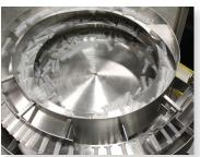
• Bowl Feeder Custom-designed specifically for the part — flows directly into the print production line smoothly and efficiently. Sorts, orients and feeds parts for printing.
