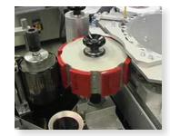
**Rotary Pad Printer** has a drum-shaped pad that rotates with an opposing drum-shaped etched cliché. Ideal for vertical or horizontal printing on syringes.
