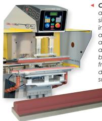
Custom pads are available in any length, size and shape. It is important to choose a pad shape that will achieve a "rolling" action when the ink is both picked up from the cliché and deposited on the substrate. Pads have
