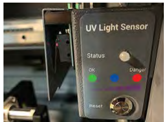
The new UV light sensor prevents accidental curing of print heads
