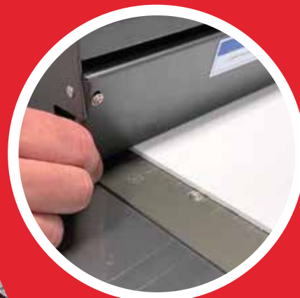
Crashbar protects printheads from damage
