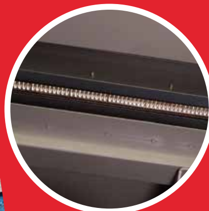
Inline, water-cooled LED curing lamps
